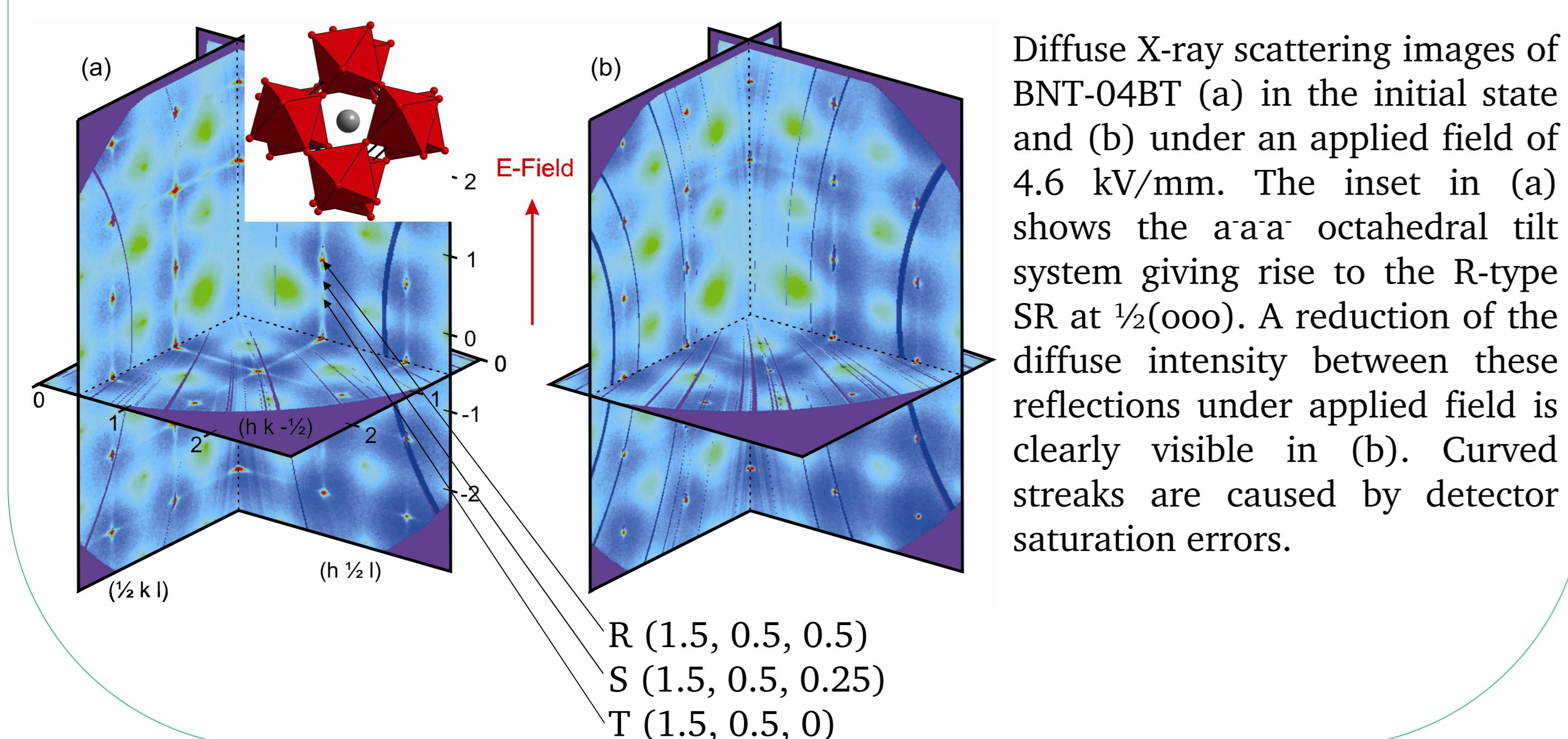
Diffuse X-ray scattering images of BNT-04BT (a) in the initial state and (b) under an applied field of 4.6 kV/mm. The inset in (a) shows the a-a-a octahedral tilt system giving rise to the R-type SR at  $\frac{1}{2}(ooo)$ . A reduction of the diffuse intensity between these reflections under applied field is clearly visible in (b). Curved streaks are caused by detector saturation errors.
