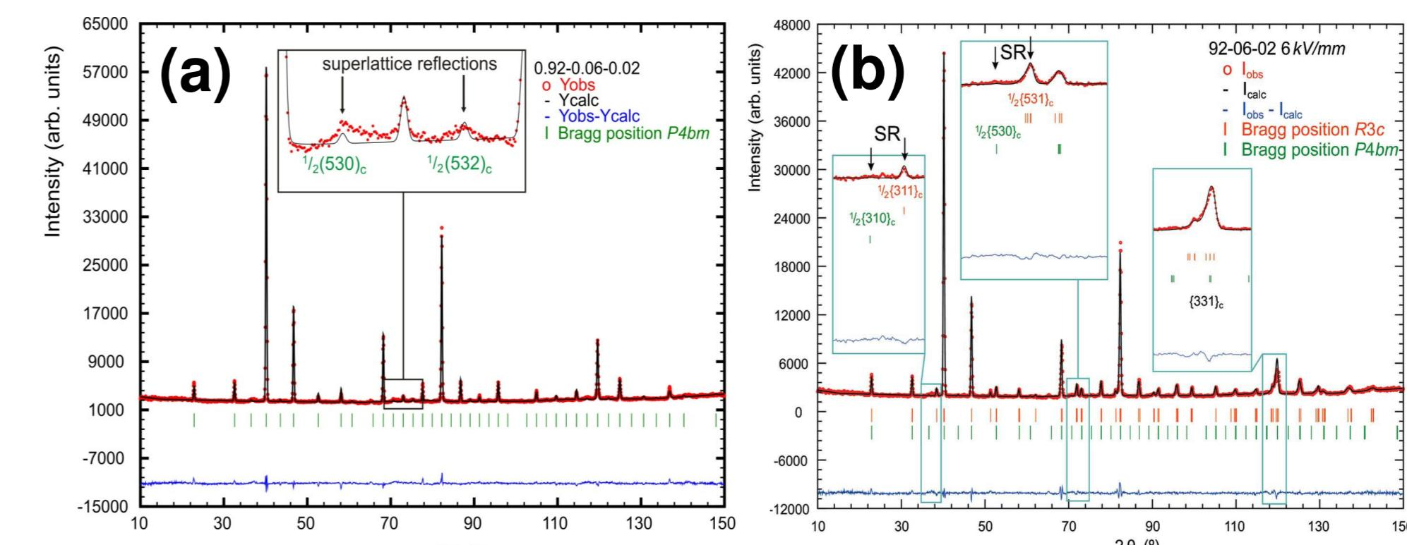
Rietveld refined neutron diffraction data of sample 92-06-02. (a) In the initial state  $\frac{1}{2}(ooe)$  SR are present. (b) Under an electric field a phase transformation from the tetragonal P4bm to the rhombohedral R3c phase occurred.
